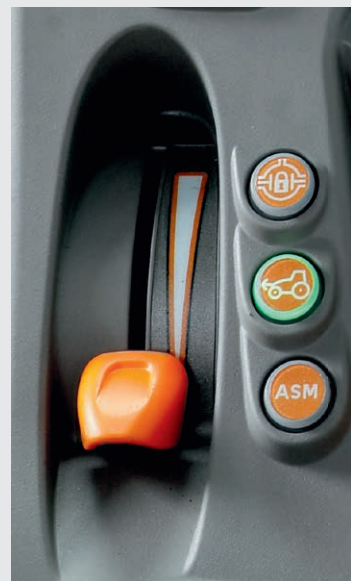
↑ Electro hydraulically operated 4WD and differential lock including ASM.
