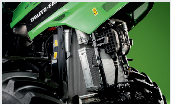
↑ Easy radiator and air-filter access.
