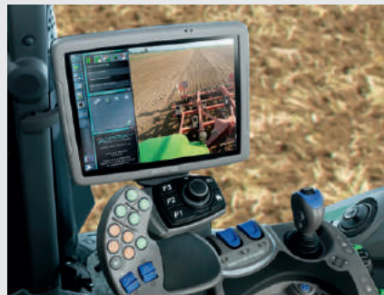
↑ Integrated camera with automatic full screen mode (e.g. reversing) for a clear overview and safety.
