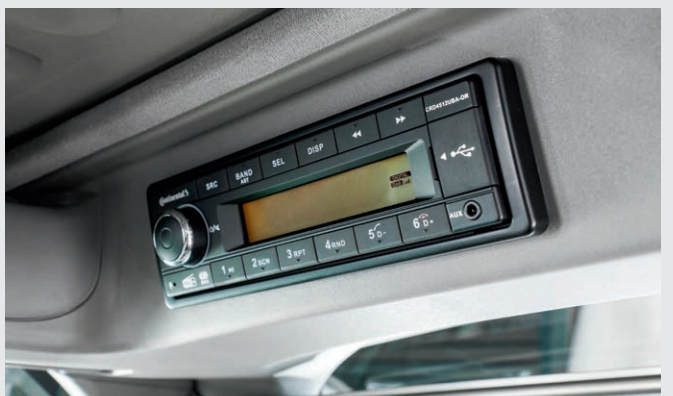
↑ New DAB+ radio with four loudspeakers and handsfree funktion, integrated into the InfoCentre Pro .
